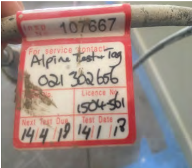
Expired test tag – painter's light
