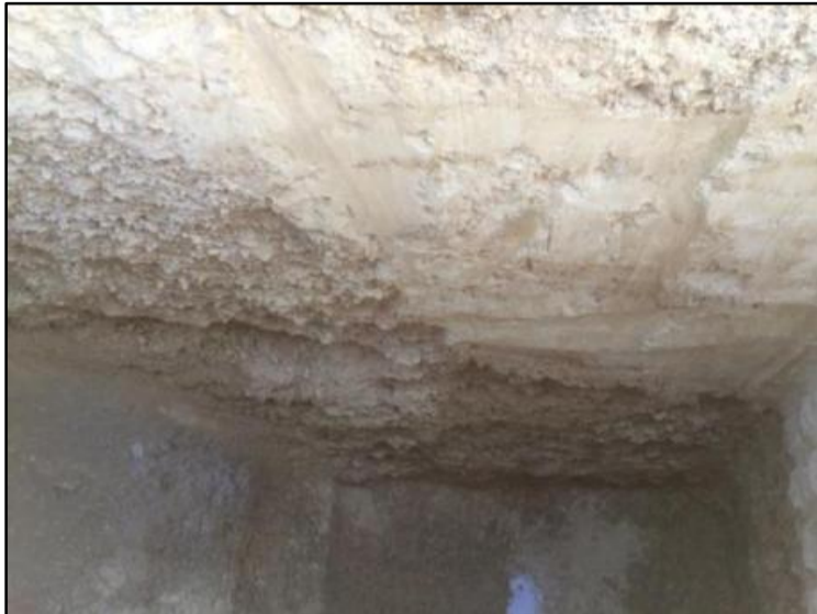
Photo 1: View of the soil profile (west face) of TP 101. On the right hand side of the photo is a sand dominated soil while the left is a gravel dominated soil. Likely a historical flow path
